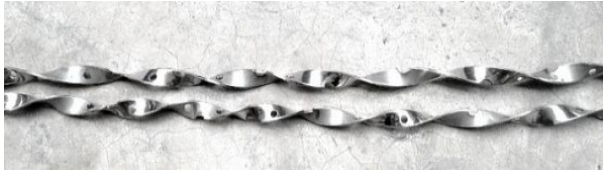
Fig 2.1: Double counter twisted tapes
